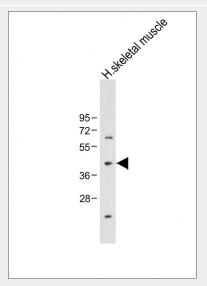
Anti-ADIPOR2 Antibody (Center) at 1:1000 dilution + Human skeletal muscle tissue lysate Lysates/proteins at 20  $\mu$ g per lane. Secondary Goat Anti-Rabbit IgG, (H+L), Peroxidase conjugated at 1/10000 dilution. Predicted band size : 44 kDa Blocking/Dilution buffer: 5% NFDM/TBST.
